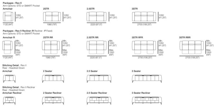
Effective June 2022. Reo II Recliners use TouchGlide® Technology. The weight limit for the recliner mechanism used in Reo II Recliners is 120kg (264.5lb). The weight limit for Reo II Recliner footrest is 15kg (33lb). Reo II Recliners have support legs (Reo II Armchair Recliner excepted). King has a policy of continuous improvement, changes to products and specifications may be made without prior notice. Images and drawings are representative of design only. Accessories not included.
